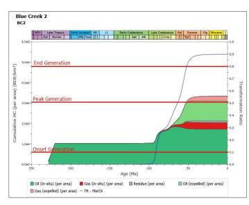
Transformation Ratios show that the earliest phase of generation occurred between 100 Ma and 90 Ma during the deposition of the Yalbac formation and was limited to the north-western portion of the Corozal basin. The second phase of generation was more diffuse, and occurred between the onset of Barton Creek deposition (80 Ma) and the end of El Cayo deposition (53 Ma).
