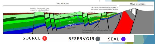
Geological Cross Section Across the Corozal Basin Showing the Petroleum System Elements
