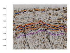
Seismic Section Across the Never Delay Oil Field in the Corozal Basin showing Trap Associated with a Possible Inversion Structure
