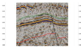
Seismic Section Across the Spanish Lookout Oil Field in the Corozal Basin showing Footwall Trap in a Tilted Fault Block
