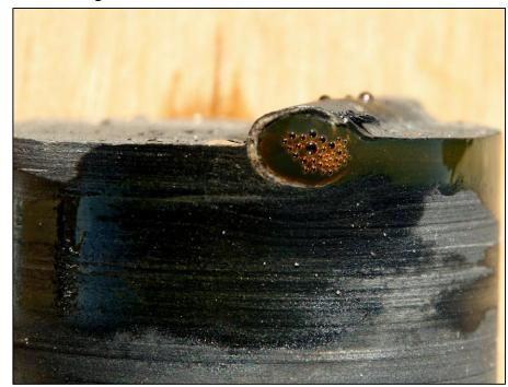
Carbonate-filled fracture with oil stains. Blokely core, Jameson Land
